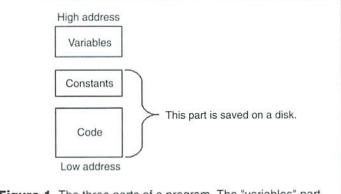
Figure 1. The three parts of a program. The "variables" part doesn't need to be saved on disk, since values will be set up as the program runs.
