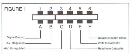
The Cassette port edge connector. Upper and lower pins are shortened. Note that this connector is keyed between pins 2 and 3.
